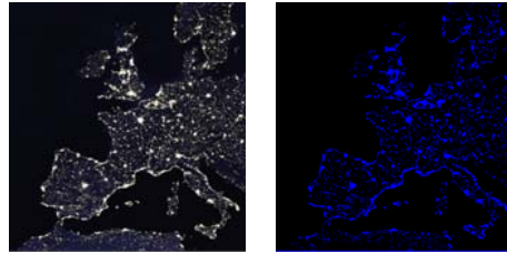
Fig. 3: Left: the original image of "Europe-at-night". Right: CVT-based segmentation into two clusters.
