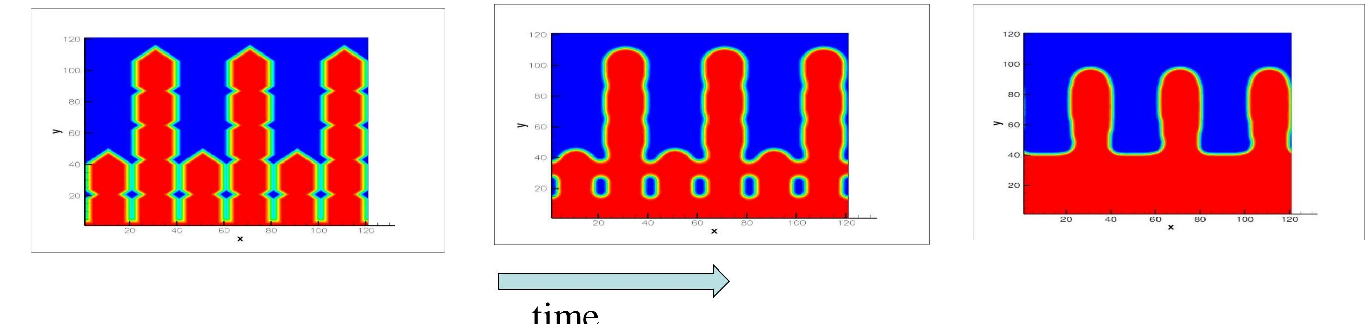
The feathery (Saw-tooth) structure smooth out very fast and the necks form between the columns then the material continue to transport from the top to bottom faster.
