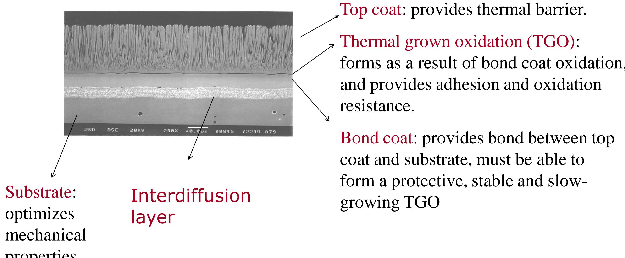
The common substrates are nickel based alloys whereas as the common topcoat is yttria-stabilized zirconia(YSZ). So there is a thermal expansion mismatch that we should take it into account in the model
