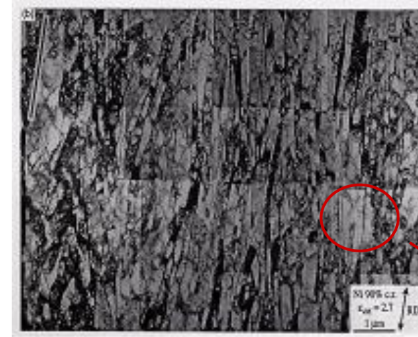
Resolved region showing complex dislocation structure
